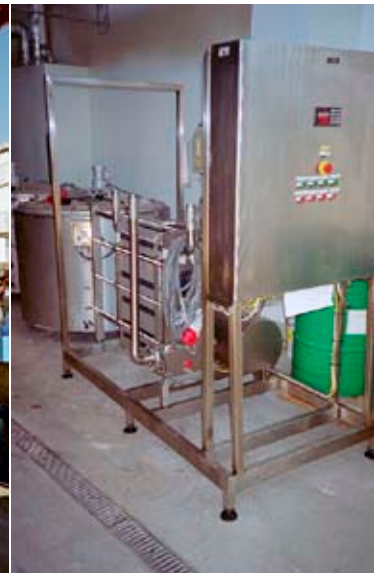
Delivery of new wort cooler module from Maseco to Fruängskällan
